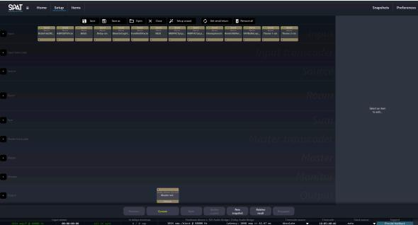
Select all the objects in the 'empty' signal graph using a drag select or Command click selection, then choose the 'connect selected' action. A default module routing will be completed automatically with a default stereo virtual room.
