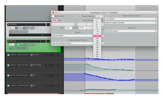
First, set up a Track in Reaper that can handle 16 channels simultaneously. Then add a SPAT RETURN plug-in on this track. It should automatically inherit the channel count, if not do it manually using the IO config of the plug-in, available from the little cog wheel in the top corner of SPAT RETURN.
