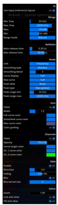
Copyright (c) 2023 FLUX:: SE, All Rights Reserved. Figure 15.5: Magnitude spectrum setup dialog Display range can be switched from a fixed reference interval to one that automatically adjusts to the current range of spectrum magnitude values. The latter is useful as a set and forget setting and works well to display the most vertical detail, at the expense of losing the ability to visually compare the current values to a reference level.
